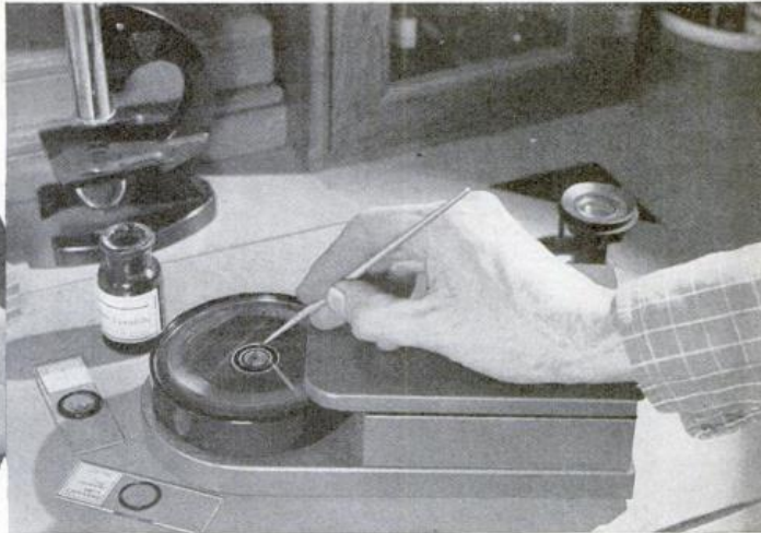
A ring of shellac being built up on a microscope slide with the aid of the turntable. The disk is spun by hand, and shellac is applied with a small, artist's painting brush
